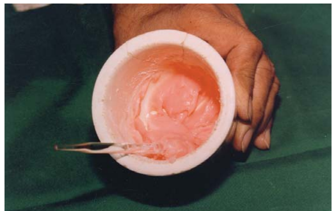
Fig. 10.5: "Wet-sand" stage of acrylic denture base material
