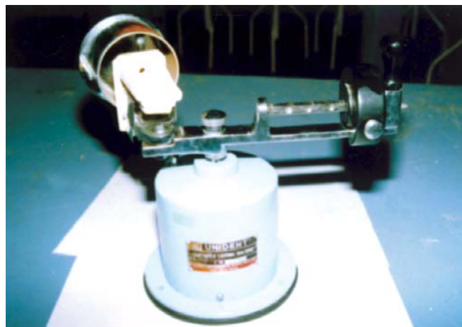
Fig. 20.12: Centrifugal casting machine (Broken-arm type)
