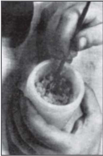
Fig. 10.6: Mixing acrylic resin "wet sand" stage
