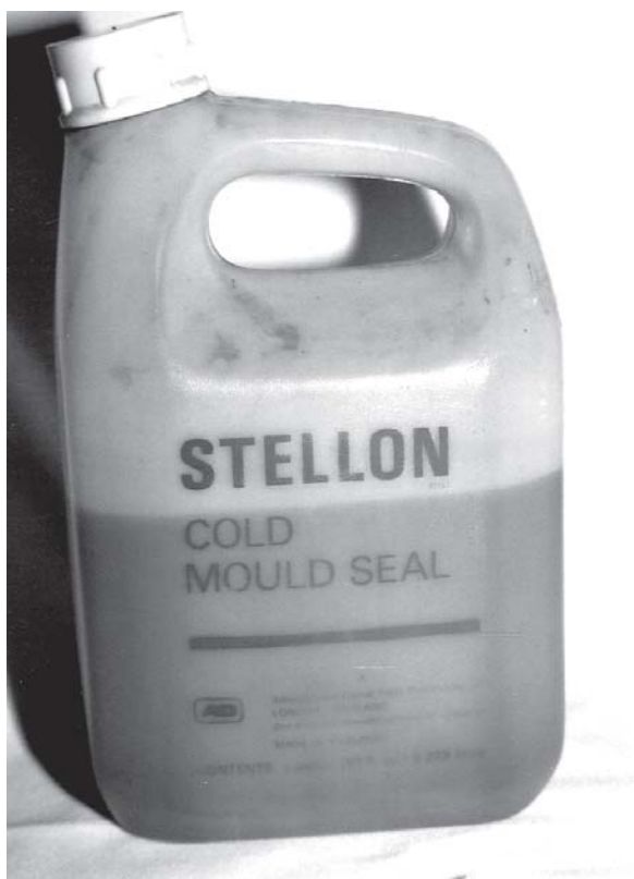
Fig. 10.4: Separating medium. Cold mould seal
