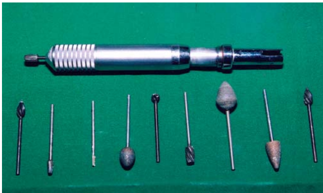
Fig. 10.17: Denture finishing instruments Laboratory straight handpiece Assorted burs and stones
